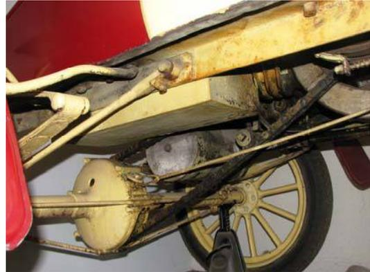
lettered model A, then model B, etc. until the Model T proved so popular that Ford kept producing that Model T for several years. Then Ford went back to producing a new Model A. As the picture at right shows, the 1903 Ford Model A was chain-driven. The car often had the problem of mud, etc. clogging up the operation.<sup>8</sup>
